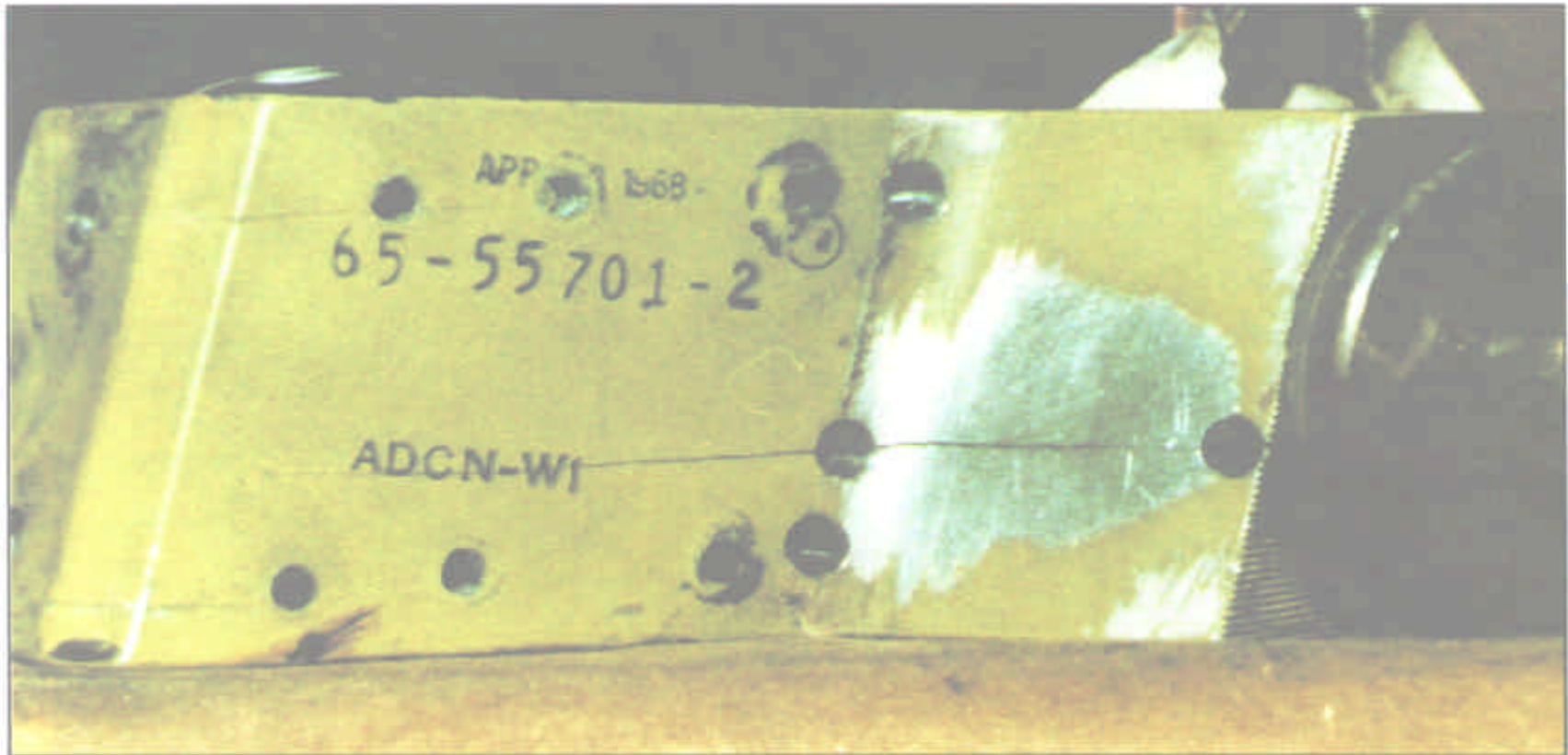
FIGURE 2-12. STRESS-CORROSION CRACKING OF 7079-T6 FITTING
