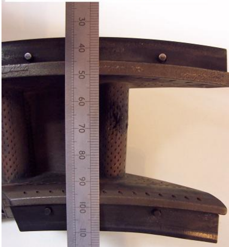
CFM56-3 HPT nozzle, scale in mm
