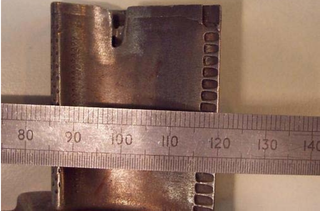
CFM56-3 HPT blade, scale in mm
